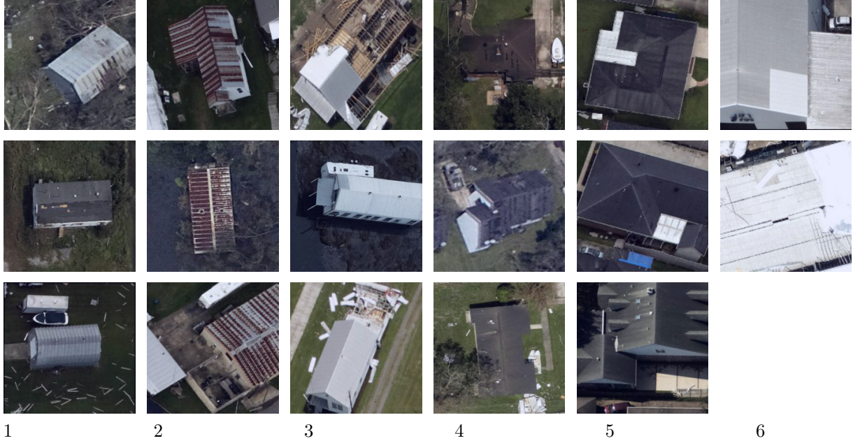
Figure 4: Building types by column. 1: Small outhouses and informal buildings. 2: Corrugated-iron roof shotgun-style houses. 3: Wooden roof shotgun-style houses. 4: Medium residential houses. 5: Larger residential houses. 6: Large commercial buildings.
